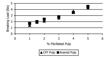
Disc Pad Preform Stiffness CFF Pulp vs. Aramid Pulp
